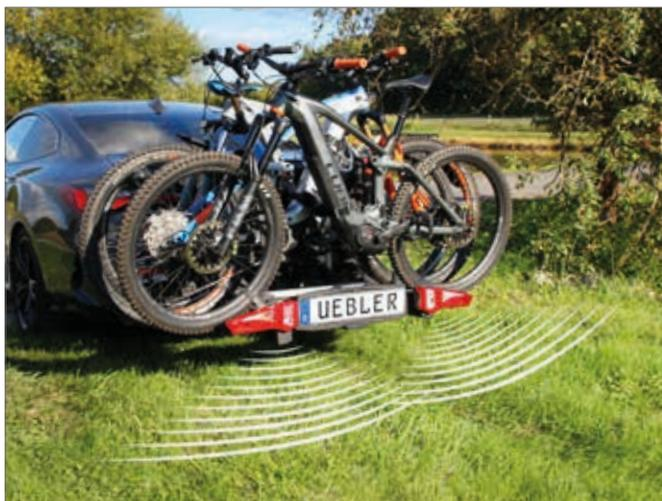
These innovative carrier systems with the integrated Distance Control (DC) parking aid at the highest Uebler standard combine all the advantages of the respective products with additional convenience when reversing and parking. Obstacles are detected unerringly and are indicated visually and acoustically.
